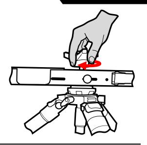
8. Turn the handle to control ball-joint of the bench.
