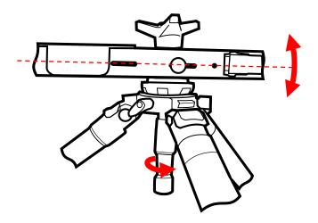
9. Open the wings to the desired position.
